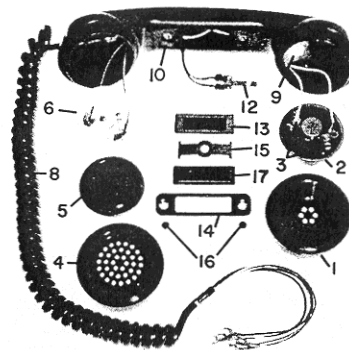
Fig. 4-1 COMPONENT PARTS - EXPLODED VIEW
